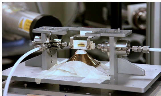
Fig. 1 The adsorbent bed, in place on the B18 EXAFS beamline at Diamond. The stage was moved in 1 mm steps to enable data collection at five positions along the adsorbent bed.
