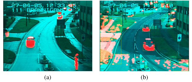
Fig. 8. MoG motion detection algorithm on GPU. (a) Motion bounding boxes successfully identified. (b) False positives due to illumination changes and camera shake.
