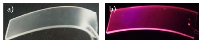
Figure 5. Photographs of the hydrogels encapsulated with 1.Eu and swelled in deionized H 2 O. Images were captured a) under ambient light and b) upon irradiation at 254 nm.
