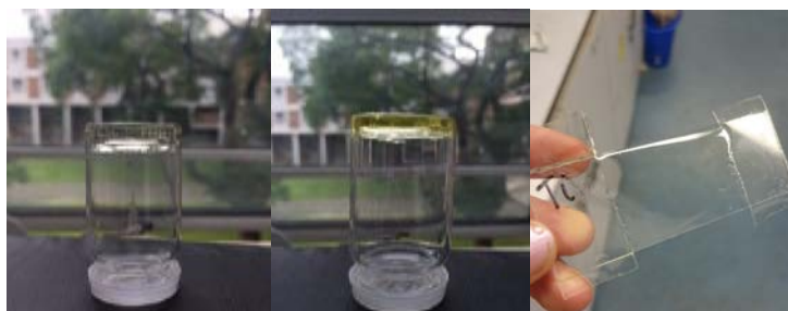
Figure 1. (a) SiO 2 [P 66614 ][OH] gel (b) TiO 2 [P 66614 ][OH] gel (c) TiO 2 Film (cast).
