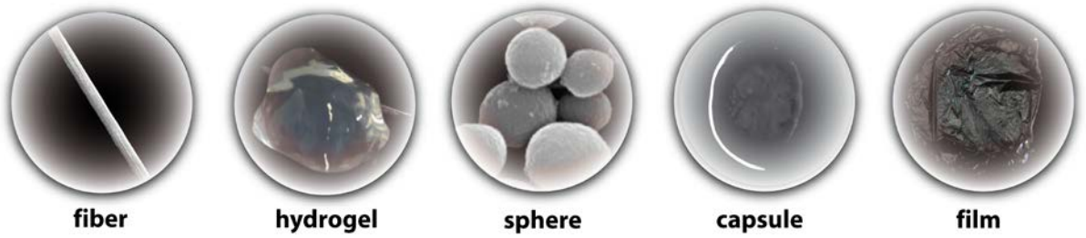
Figure 4. The various morphologies that we have prepared with our bioengineered silk proteins.
