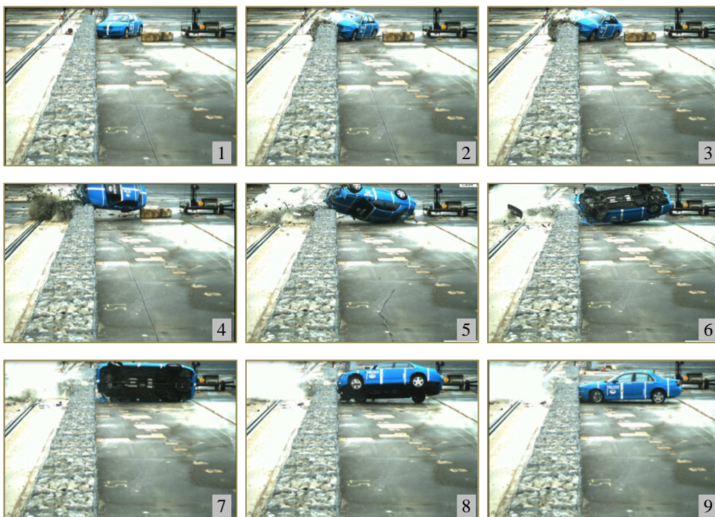
Figure 11. Gabion specimen type D at 60 ms from the impact start.
