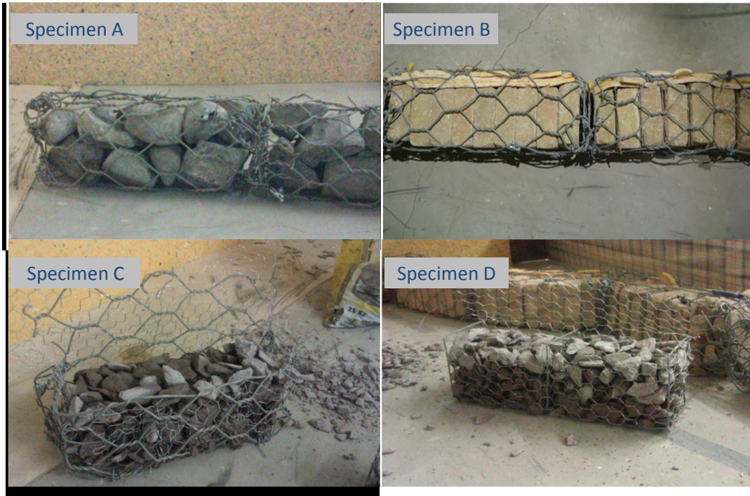
Figure 9. Gabion specimen types A-B-C-D.
