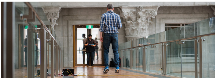
Fig. 14. Jumping on Skybridge SB4 with IMUs attached to jumper C7 and deck at midspan.
