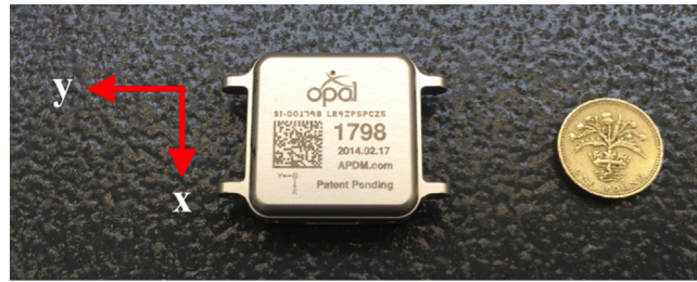
Fig. 1. APDM Opal™ inertial measurement unit showing local coordinate system (LCS) axes; +z is vertical, upwards. A one-pound coin is shown for size reference.
