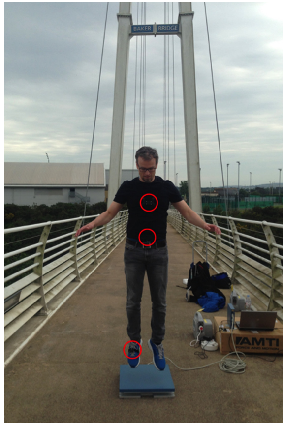
Fig. 10. Jumping test at Baker Bridge. Second author is instrumented with IMUs at sternum, navel, lower back and C7 (not visible) and right foot; the bridge is instrumented with IMUs and a force plate. The collection of equipment around the cardboard box is necessary to operate the force plate.
