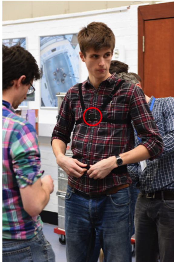
Fig. 7. Instrumenting a student with IMU on sternum (circled), and lower back.
