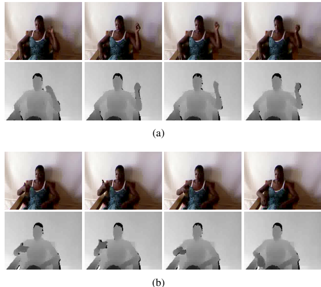
Fig. 6. Examples of challenging gestures. (a) An example of a gesture where RGB information is capable of recognising the gesture while depth information fails. (b) An example of a gesture where depth information is capable of recognising the gesture while RGB information fails.
