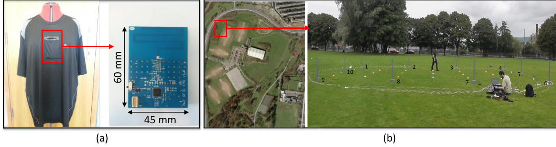
Fig. 1. (a) Purposely developed garment with mounting pocket at front central chest and the bodyworn wireless node used in the measurements; (b) satellite view of the measurement environment showing the positions of base stations.
