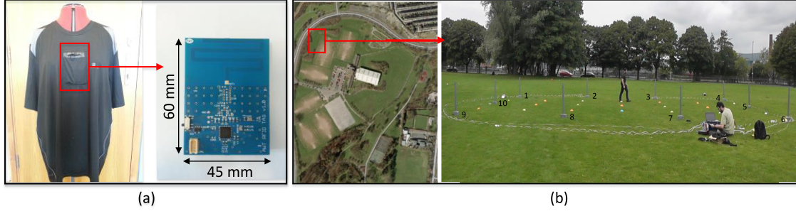
Fig. 1. (a) Purposely developed garment with mounting pocket at front central chest and the bodyworn wireless node used in the measurements; (b) satellite view of the measurement environment showing the positions of base stations.
