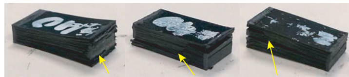
“brush”-like layer splitting shear-driven fibre fracture kink band
