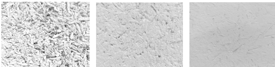
211 Figure 3. Surface finishes of (left) unfinished hemp-lime concrete, (middle) 1:1.25 lime-hemp render, (right) 2:1 212 lime-hemp render.
