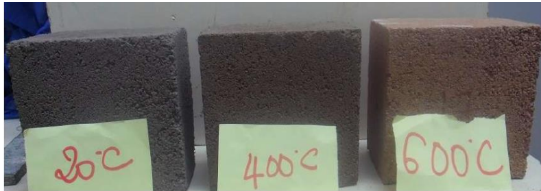
Figure 6. Brick appearance after furnace heating.
