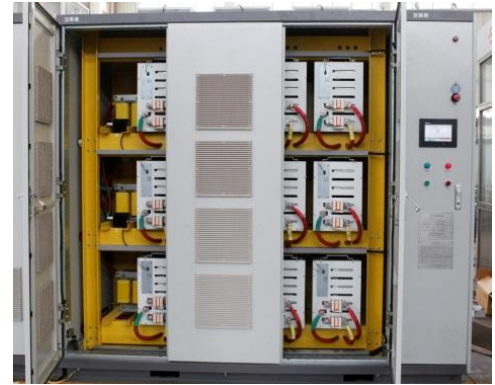
(b) Nine-level high voltage inverter
