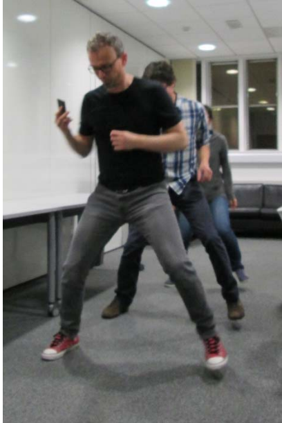
Fig. 16, three of the authors stepping laterally to a predetermined beat on the 7 th floor to excite building motion.
