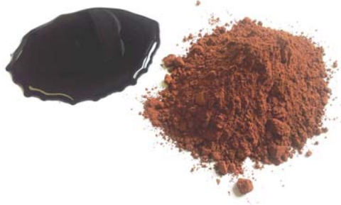
Figure 1: Liquid activator and powder component produced by banah UK Ltd.
