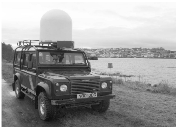
Figure 2: Ground Trials Vehicle, with PMMW imager in radome
