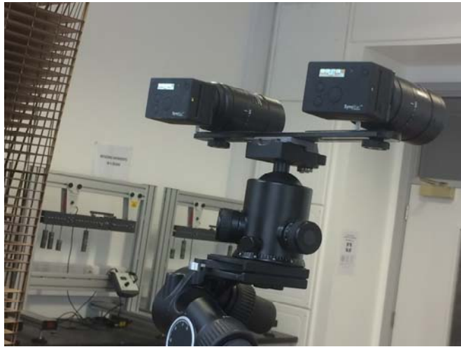
Fig 2 Camera mounting configuration for laboratory and field trials
