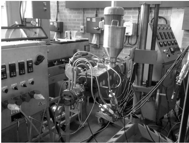
FIG. 5. Photograph of the laboratory Killion KTS-100 single screw extruder with in-line-rheometer die.
