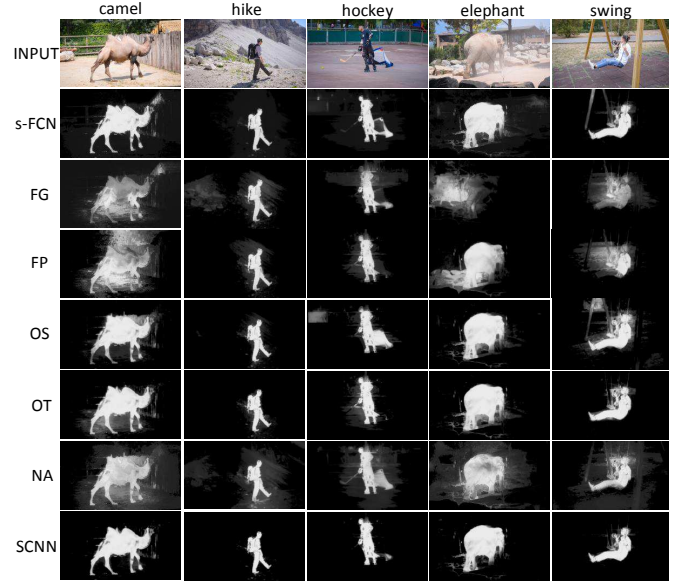
Fig. 8. Saliency maps by different configurations. From top to bottom, they are saliency maps by single FCN (s-FCN), connecting graying optical flow prior map and spatial prior map (FG), connecting spatial prior map and temporal prior map (FP), only using the spatial prior of video frame (OS), only using temporal prior map (OT), saliency maps without weak pixel-wise labels (NA) training and Final saliency map (SCNN) with all of components
