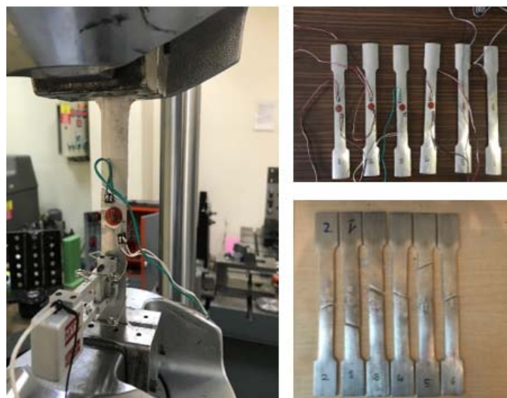
Figure 1: Tensile test specimens of AL6063 aluminum alloy.
