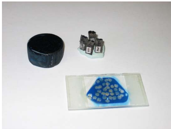
Figure 5: Example of FRP microscopy sample prepared from representative batch specimens
