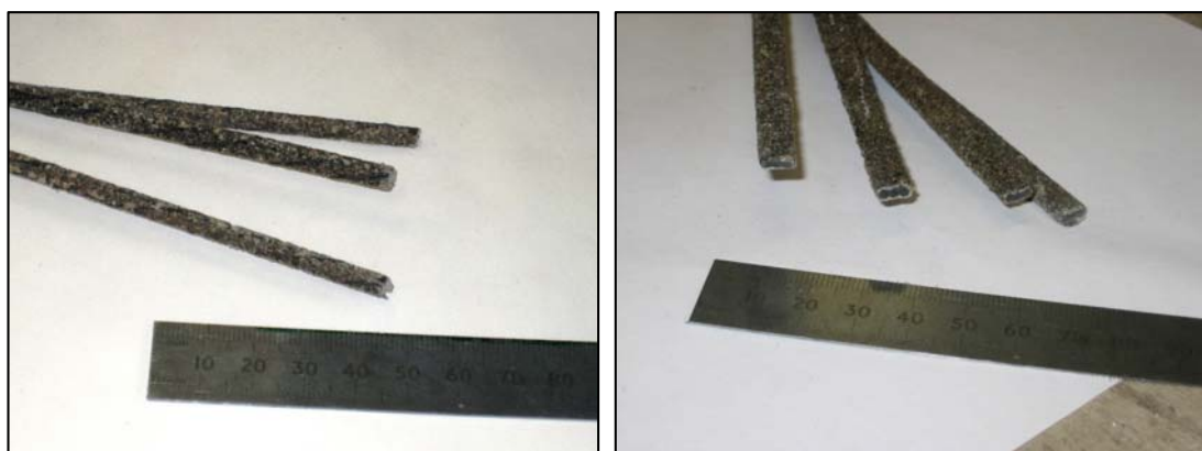
Figure 5: Example of FRP microscopy sample prepared from representative batch specimens
