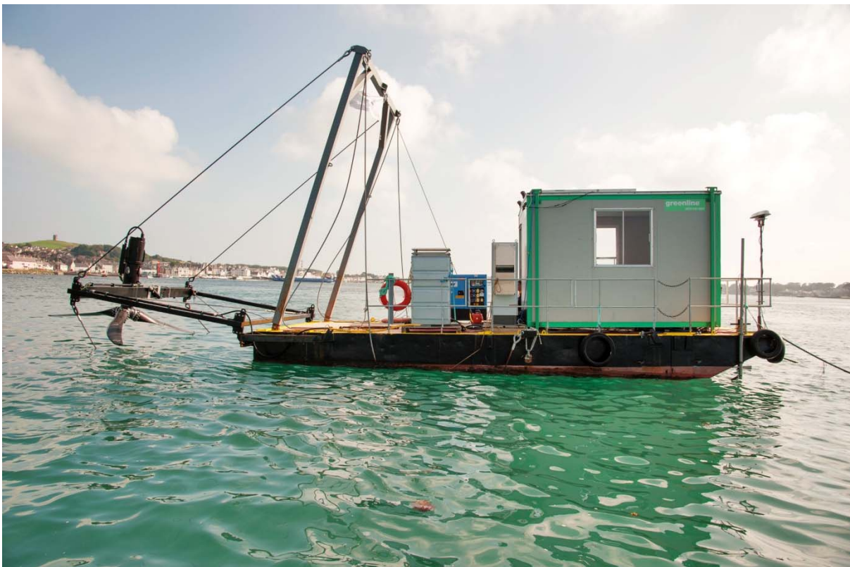
Figure 8: Barge with turbine in lifted position
