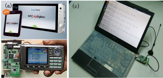
Fig. 4. (a) The world's first Android tablet PC integrated with ZigBee radio [34]. (b) The world's first mobile phone integrated with a ZigBee interface produced by Pantech&Curitel [30]. (c) A laptop client with a ZigBee interface via a USB interface in our testbed.
