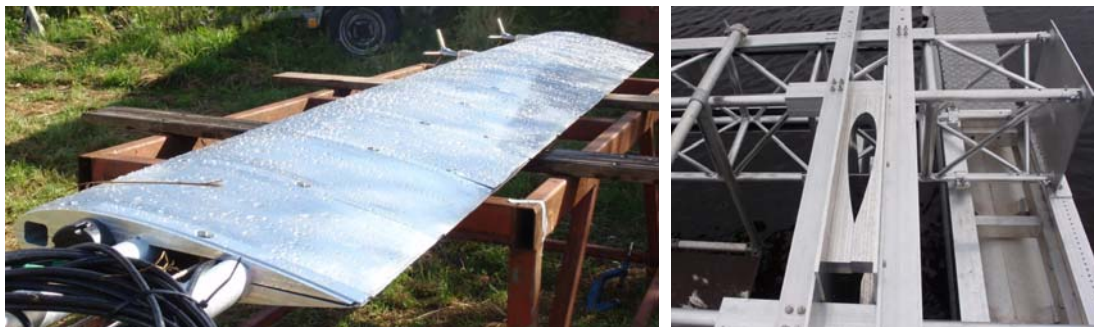
Figure 7: Assembled hydrofoil strut (left), hydrofoil clamp in place on the towing rig (right).
