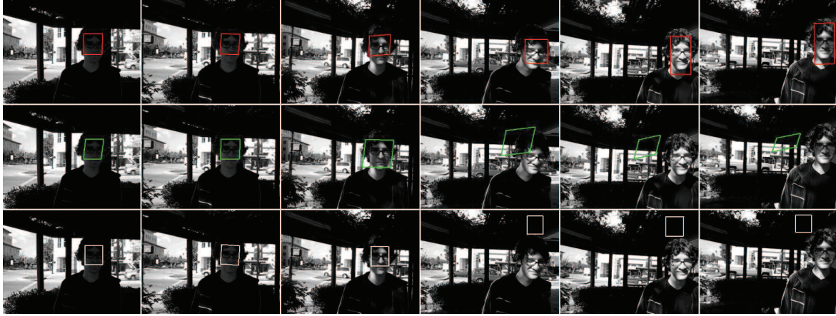
Figure 6: The tracking results of the head sequence with significant pose, lighting and scale variation in a cluttered scene. The first, second and third rows are results obtained by the proposed method, L1 tracker and IVT tracker, respectively.
