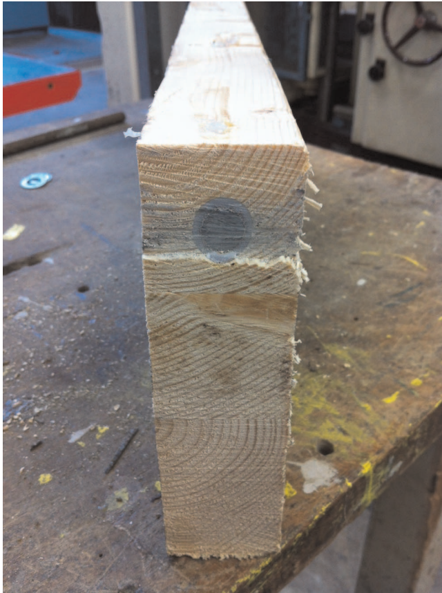
Figure 2. Results of adhesive testing to ensure sufficient bond is achieved
