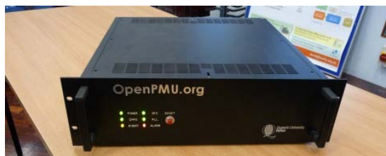
Fig. 2. The OpenPMU unit in 19" rack form factor enclosure.
