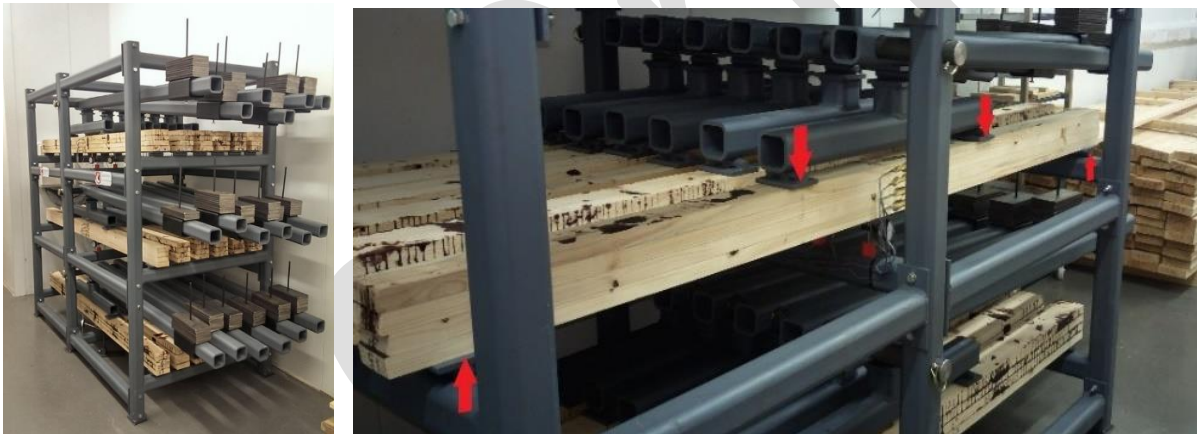
222 Fig. 4. Creep test frame: (a) Loaded creep test frame in a constant climate condition at a temperature of 20 \pm 2 °C and at a relative 223 humidity of 65 \pm 5\% , (b) Creep test beam loaded in four-point bending.
