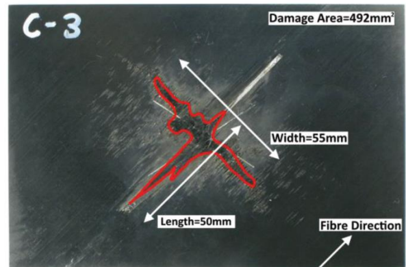
Moderate and severe damage areas for 7/150 \mu s, 10 kA specimen
