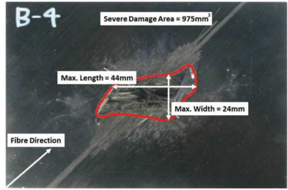
Moderate and severe damage areas for 4/20 \mu s, 40 kA specimen
