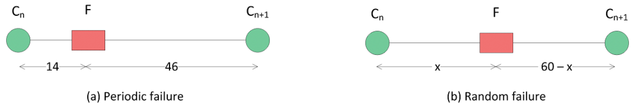
Fig. 16. Fault occurrences between two checkpoints, C_n and C_{n+1} . (a) Periodic failure that occurs 14 minutes after C_n and 46 minutes before C_{n+1} . (b) Random failure that occurs x minutes after C_n and 60 - x minutes before C_{n+1} .
