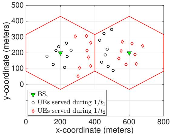
Fig. 10: Users in a twin-cell network under Scenario 3.
