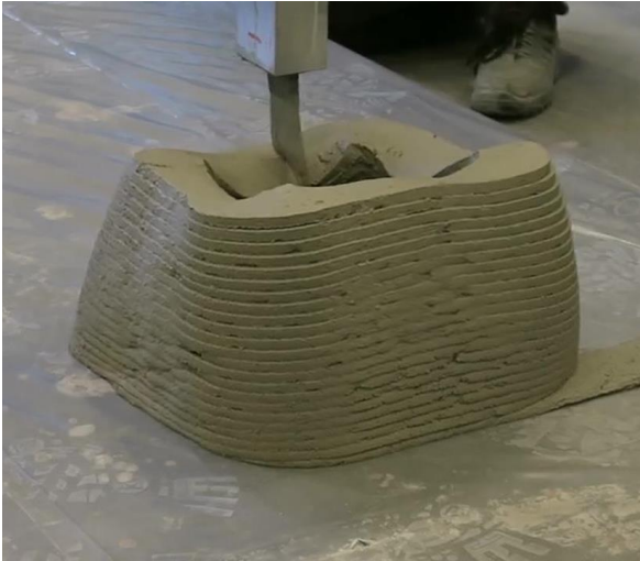
a) b) Figure 6. Collapse in extrusion-based additive manufacturing: a) material failure, b) stability failure [60].
