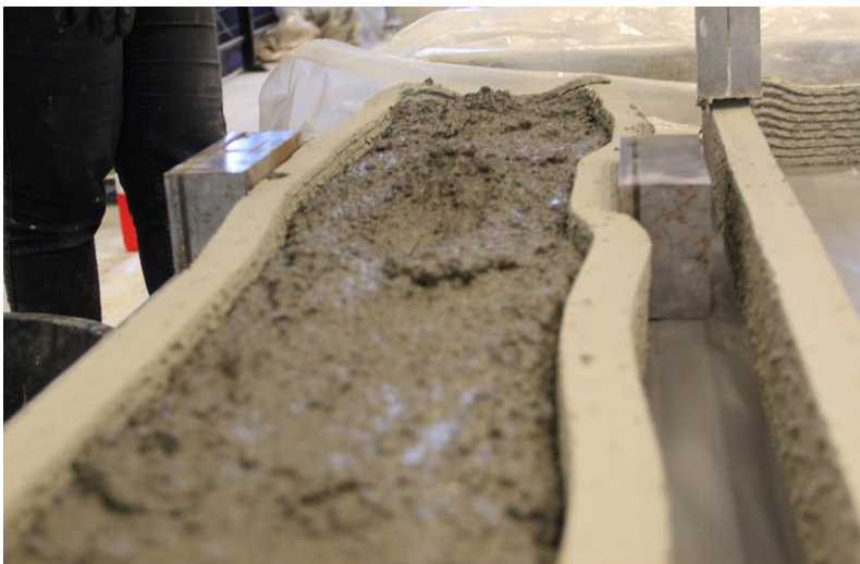
Figure 7. Structural failure of an object during 3D printing due to horizontal loading by a highly fluid infill material
