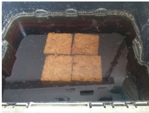
182 Figure 3.1 – Rapeseed VMA samples during an immersion weathering test
