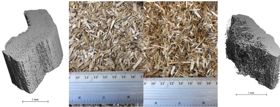
113 Figure 2.1 – Photograph and X-Ray tomography image of aggregates used in this investigation, 114 hemp shiv (left) and rapeseed straw (right)
