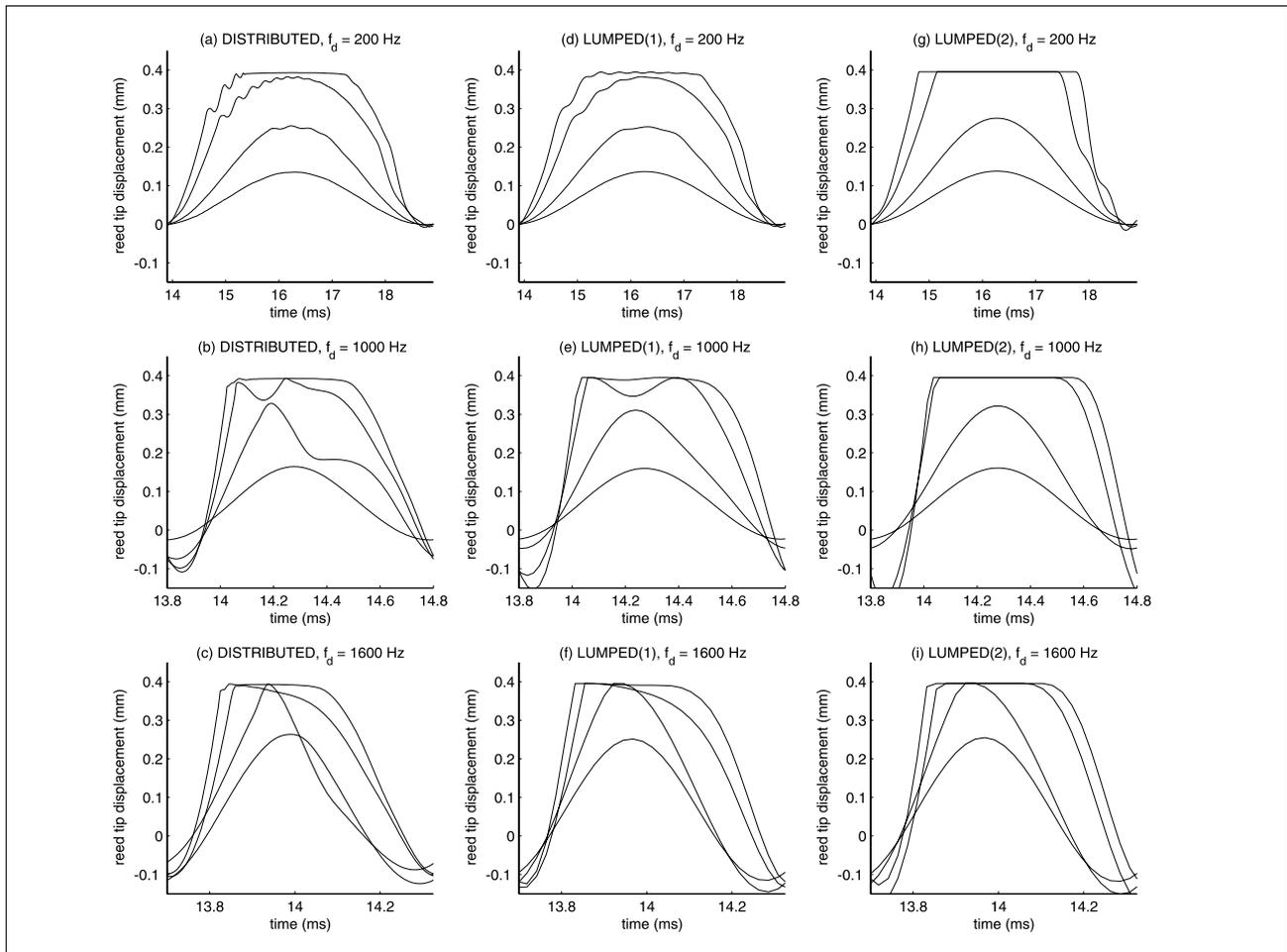
Figure 6. Steady-state comparison between the distributed model, the lumped model with pressure-dependent  $K_a$  [lumped (1)], and the lumped model with abrupt beating [lumped(2)], for different driving frequencies and amplitudes. For each driving frequency, exactly one period is plotted.
