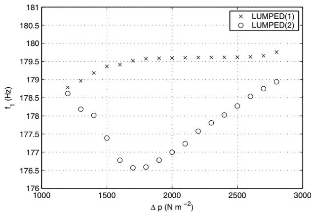
Figure 9. Playing frequency as a function of mouth pressure. All data-points were calculated using FFT-analysis of the waveforms obtained by running the simulation with a constant mouth pressure. Plotted are the results obtained with the lumped model with pressure-dependent stiffness per unit area [lumped(1)], and with the lumped model with abrupt beating [lumped(2)].
