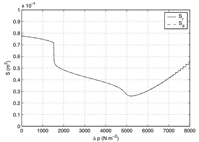
Figure 4. Effective surface as a function of pressure difference, as derived from static simulations with the distributed model. Note that the curves of  $S_r$  (solid) and  $S_d$  (dashed) almost entirely overlap.
