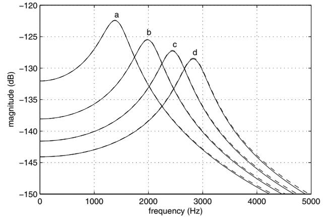
Figure 2. Reed frequency response, for 4 different values of effective stiffness. For the curves a, b, c, and d, the respective values are  $K_a = 4, 8, 12,$  and  $16 \text{ MN m}^{-3}$ . The solid lines indicate the analog responses, and the dashed lines indicate the digital responses. A 44.1 kHz sample rate was used. The y-axis displays the magnitude on a logarithmic scale, that is calculated as  $20 \log_{10}|H(f)|$ , where  $H(f)$  is the complex frequency response at frequency  $f$ .
