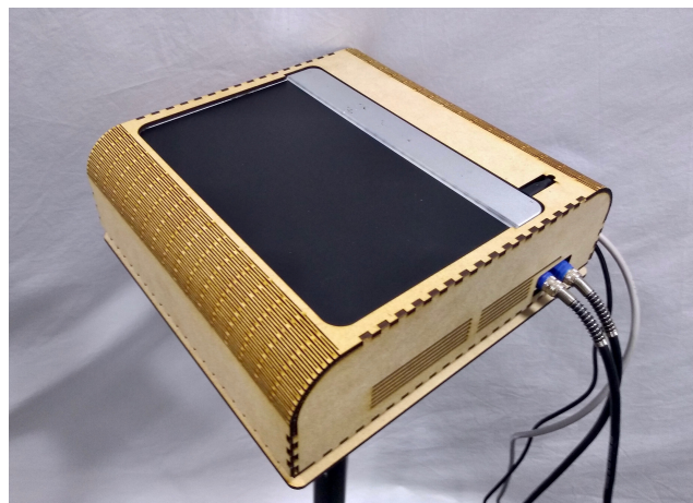
Figure 1: Vodhrán with Sensel Morph interactive surface.
