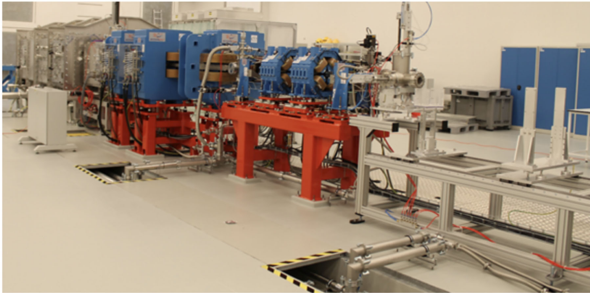
FIGURE 1 | ELIMED ion beam line connected to the Interaction chamber (first chamber from the left), where the laser-acceleration occurs and where the collection systems sits. It follows the ESS and the beam shaping section. After this last section, the beam is delivered in the in-air dosimetry station.
