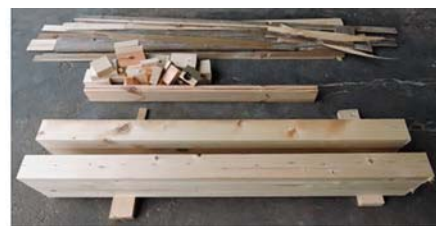
b) Glulam from reclaimed timber
