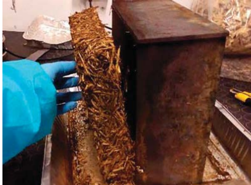
Figure 5. Insulation panel made from wood fibres.
