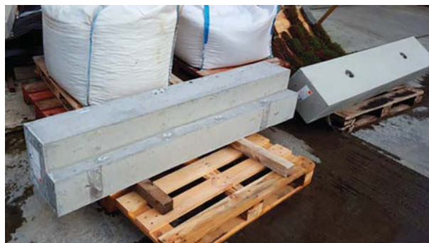
Figure 6. Precast concrete beam cast for upscaled testing.
