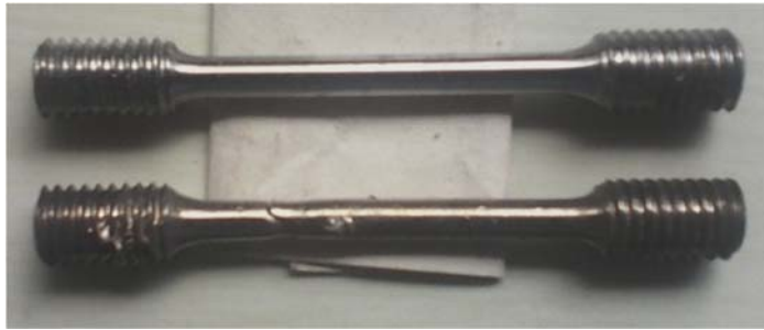
Fig. 4 Tensile specimens before and after fracture in LBE.
