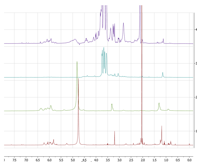
Figure 5. From top to bottom; ^1\text{H} NMR of seaweed extracts: (purple) A. nodosum crude extract, (blue) F. serratus crude extract, (green) A. nodosum after SPE, (red) F. serratus after SPE.
