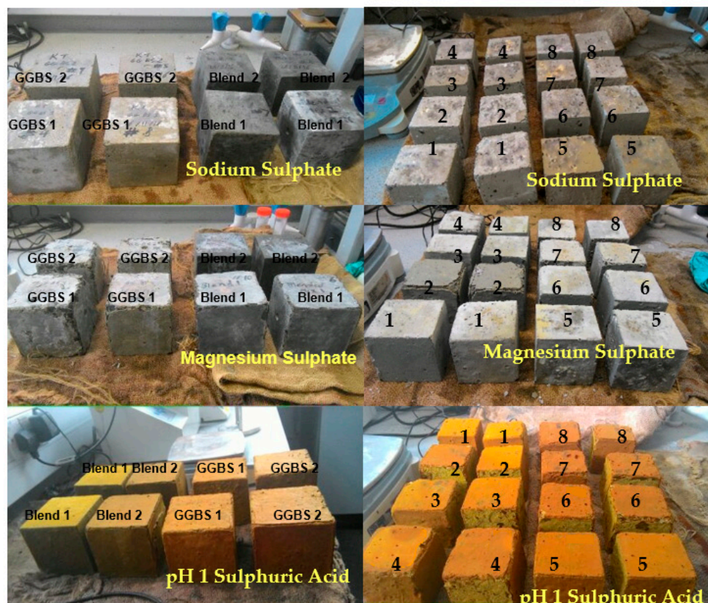
Figure 4. The visual appearance of the concrete specimens after 14 months of exposure to various solutions. Group 1 specimens are shown on the left-hand side and Group 2 on the right. The corners and edges were damaged for specimens exposed to MgSO_4 and sulphuric acid. Note the brown/orange colouration of specimens exposed to sulphuric acid.
