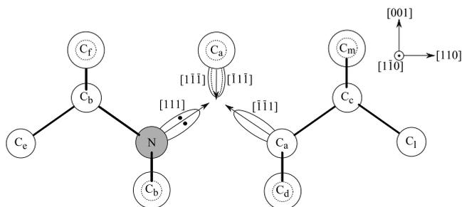
FIG. 1. Projection of the nitrogen vacancy center in diamond on the  $(1\bar{1}0)$  plane. The grey disc represents a nitrogen atom and the other circles represent carbon atoms. The larger circles represent carbon atoms located above the plane of the paper and the smaller dashed circles represent carbon atoms below the plane of the paper. The labels on the carbon atoms denote sets of equivalent neighbors.
