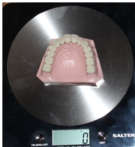
Figure 1 Digital electronic scale (Salter Housewares, Tonbridge UK) was used to measure the probing force.
