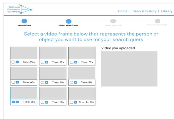
Figure 2: Wireframe of Multi-page: Select a video frame.
