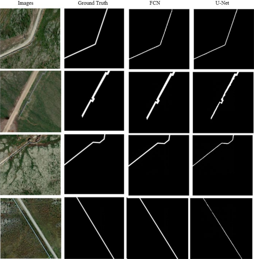
Figure 3. Experimental Results of the FCN and U-Net models. Images column indicates the actual image within the dataset, and Label column indicates the actual annotated label. The third column represents the outcomes of FCN model, and the fourth column represents the outcomes of U-Net model.
