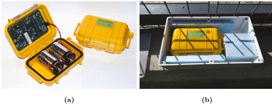
Fig. 4. Photographs showing (a) Multifunction Extended Life acceleration logger, and (b) type of weatherproof enclosure used to secure the logger onto bridge.
