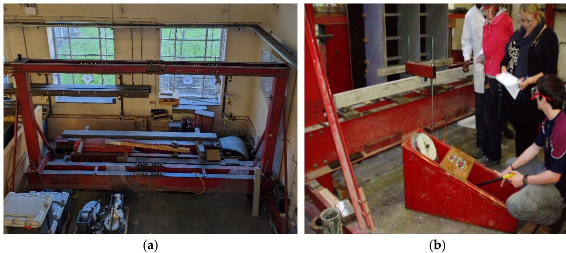
Figure 1. Arrangement of stage 1 RC beam testing experiment (a) frame for testing small capacity beams (b) hydraulic pump used to apply load to a RC beam.
