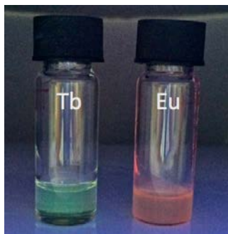
Figure 7. Visible light luminescence of [P_{666\ 14}]_3[TbCl_6] (left) and [P_{666\ 14}]_3[EuCl_6] (right) upon UV excitation (332 nm).
