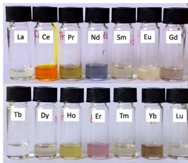
Figure 1. Samples of the room-temperature liquid rare-earth series [P 666 14 ] 3 [LnCl 6 ] (Ln = La, Ce, Pr, Nd, Sm, Eu, Gd, Tb, Dy, Ho, Er, Tm, Yb, Lu).
