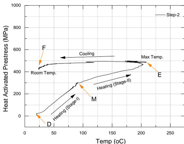
Figure 8. HAP vs temperature obtained from Test-3
