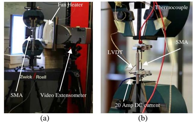
Figure 2. Test setup for thermo-mechanical tests of  $\text{Ni}_{48.46}\text{Ti}_{36.03}\text{Nb}_{15.42}$  wire specimens. (a) Video extensometer used for measuring strain; heating carried out using fan heater and heat gun. (b) LVDT used for measuring strain; heating carried out using 20Amp DC current.
