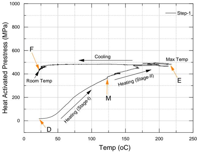
Figure 4. HAP vs temperature obtained from Test-1
