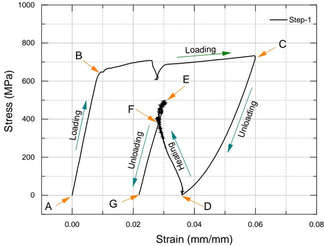
Figure 3. Stress vs strain obtained from Test-1
