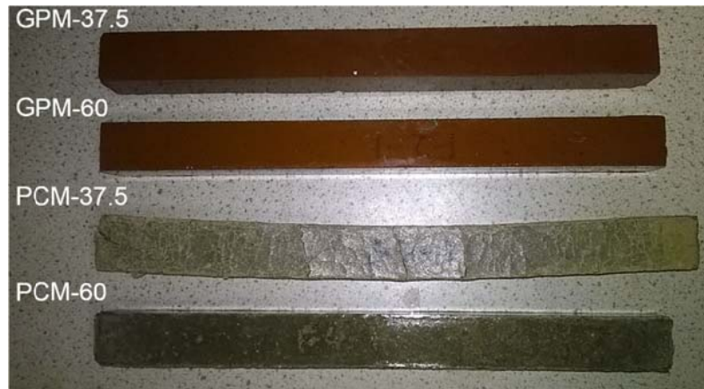
Figure 5 Samples of GPMs and PCMs after 32 weeks of exposure to \text{Na}_2\text{SO}_4 solution
