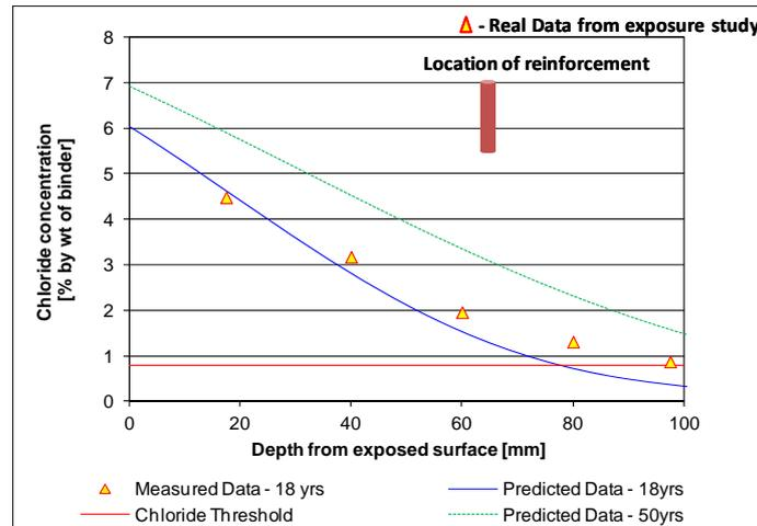
**Figure 2** Shows the real and predicted chloride concentration vs depth after 18 years of exposure and predicted chloride profile after 50 years of exposure. The 18 year data is used to validate the model before proceeding into a service life prediction for 50 years or more.
